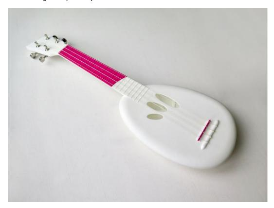
**Figure 3**Historical fagottino (wood) alongside its AM replica (white Nylon PA12). 3D model and photo by Ricardo Simian.
