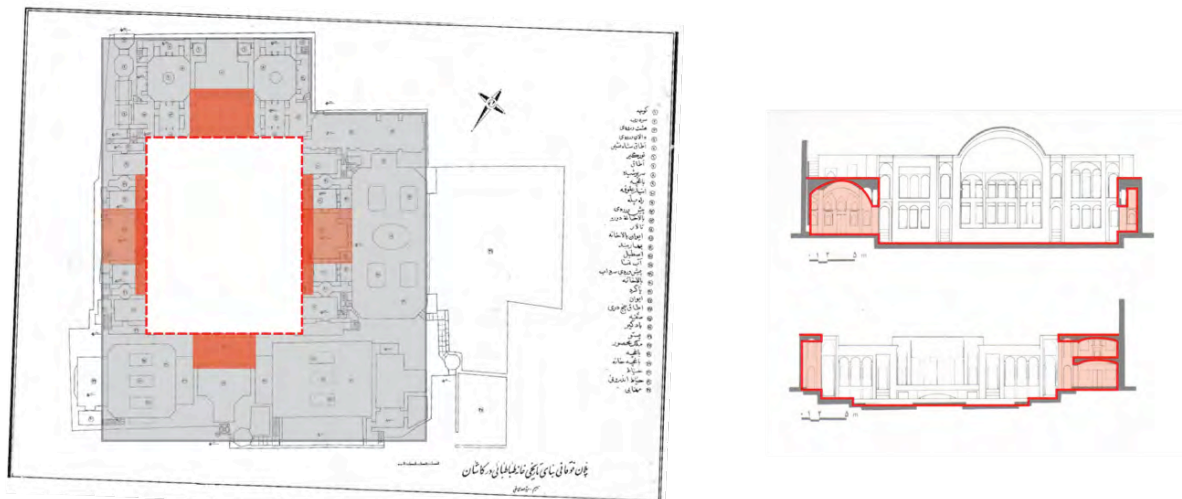
Figure 5. Semi-enclosed Iwans and the lowered courtyard setting at Tabātabāei’s house (built in the early 1880s) in Kashan, Iran. The Iwans on the north-south axis in a Persian courtyard house are usually bigger and were used for hosting guests or holding events. These Iwans usually have finer decorations than the east-facing ones.
