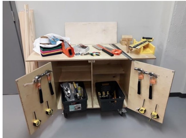
Figure 2. One product out of six from the PIPs. A movable CDT workstation facilitates working with hand tools in different, changing learning environments.
