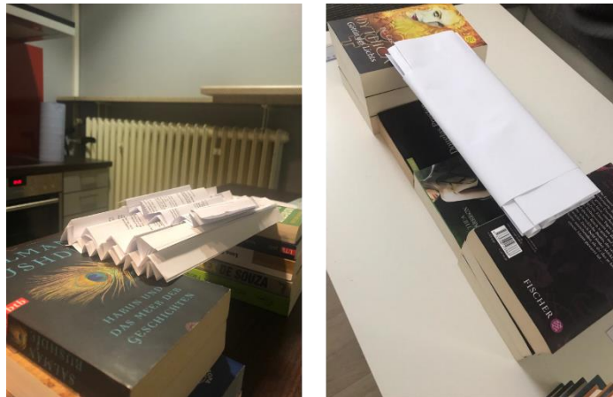
Figure 1. Bridges with maximum carrying capability (left: 3337g by expert, right: 4500g by novice)
